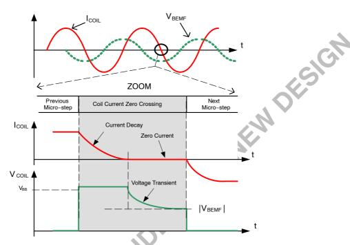
Figure 14. Principle of Bemf Measurement
