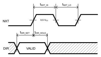
Figure 5. NXT-Input Timing Diagram
