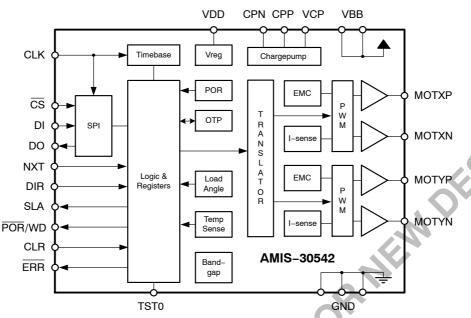
Figure 1. Block Diagram AMIS-30542
