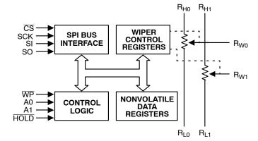
Figure 1. Functional Diagram
