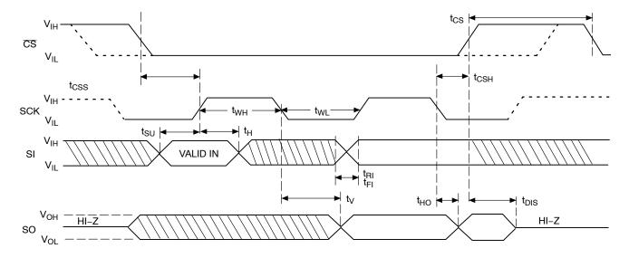
Figure 2. Synchronous Data Timing
