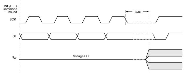
Figure 9. Increment/Decrement Timing Limits
