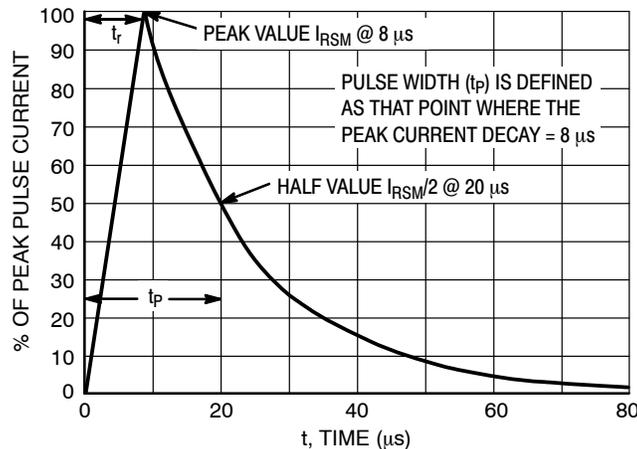
Figure 5. 8 x 20  $\mu$ s Pulse Waveform
