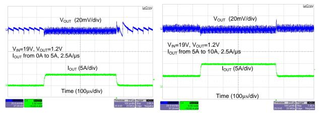
Figure 21. Load Transient from 0% to 50% Load Current
