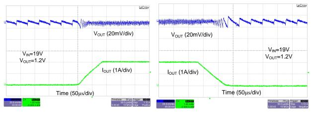
Figure 19. Operation as Load Changes from 0 A to 2 A Figure 20. Operation as Load Changes from 2 A to 0 A
