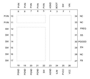
Figure 3. Pin Assignments(Bottom View)
