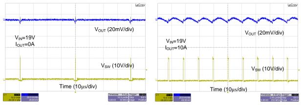
Figure 17. Static Load Ripple at Light Load
