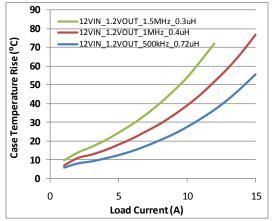
Figure 9. Case Temperature Rise vs. Load Current on Figure 10.Case Temperature Rise vs. Load Current on 4 Layer PCB, 1 oz Copper, 7 cm x 7 cm 4 Layer PCB, 1 oz Copper, 7 cm x 7 cm
