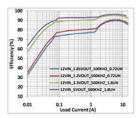
Figure 5. Efficiency vs. Load Current with  $V_{IN}$ =19 V and  $f_{SW}$ =500 kHz
