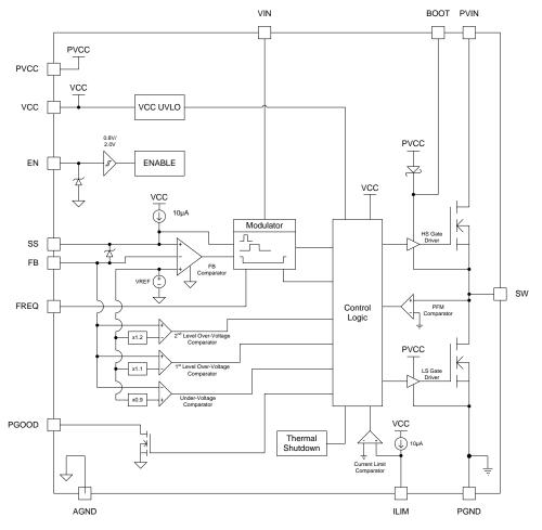
Figure 2. Block Diagram
