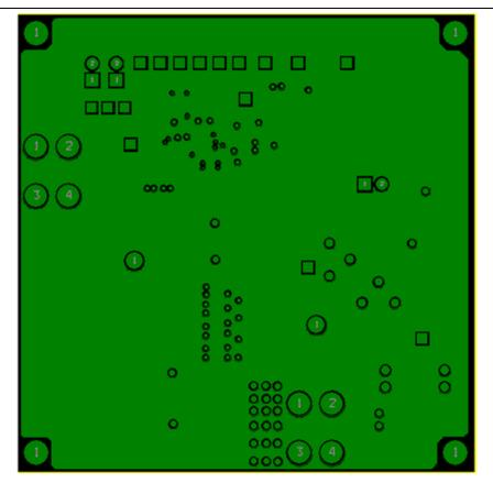
Figure 27. Evaluation Board Inner Layer 2 Copper
