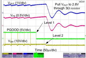
Figure 23. Over-Current Protection with Heavy Load Figure 24. Over-Voltage Protection Level 1 and Level 2
