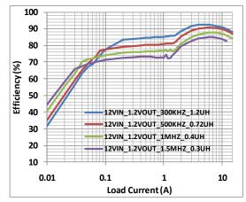
Figure 7. Efficiency vs. Load Current with  $V_{\text{IN}}$ =19 V and  $V_{\text{OUT}}$ =1.2 V
