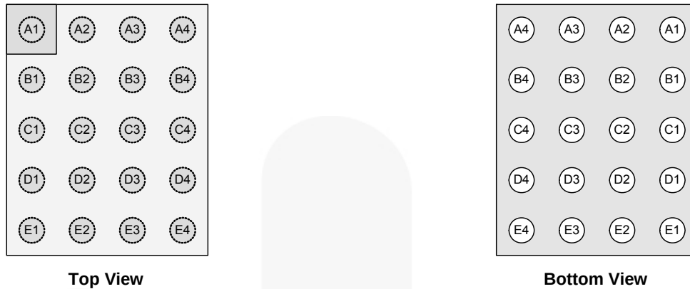
Figure 4. WLCSP-20 Pin Assignments
