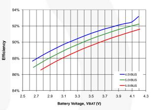
Figure 9. Charger Efficiency, No I<sub>INLIM</sub>, I<sub>OCHARGE</sub>=1,250 mA
