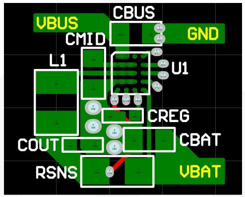
Figure 51. PCB Layout Recommendations
