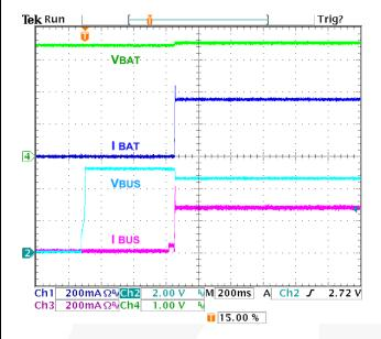
Figure 13. AutoCharge Startup with 300 mA Limited Charger / Adaptor, I<sub>INLIM</sub>=500 mA, OTG=1, V<sub>BAT</sub>=3.4 V
