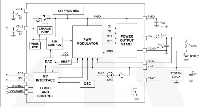
Figure 2. IC and System Block Diagram
