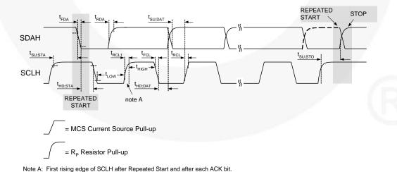
Figure 6. I<sup>2</sup>C Interface Timing for High-Speed Mode
