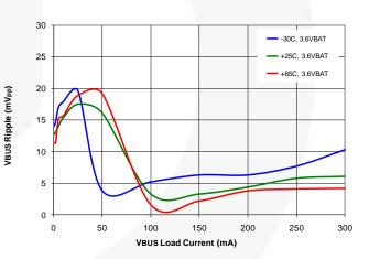
Figure 30. Output Ripple vs. Temperature
