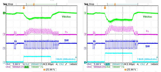
Figure 33. Load Transient, 5-155-5 mA, t<sub>R</sub>=t<sub>F</sub>=100 ns
