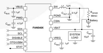
Figure 1. Typical Application (FAN5403-05 Pin Out)
