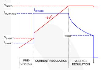
Figure 35. Charge Curve, ICHARGE Not Limited by IINLIM
