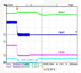
Figure 15. Battery Removal / Insertion during Charging, V<sub>BAT</sub>=3.9 V, I<sub>OCHARGE</sub>=950 mA, No I<sub>INLIM</sub>, TE=0
