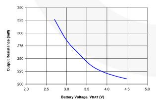
Figure 43. Output Resistance (Rout)
