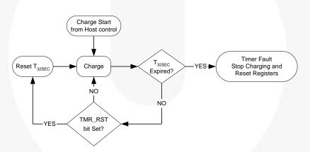
Figure 42. Timer Flow Chart for FAN5401, FAN5404
