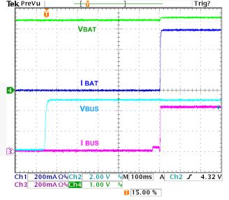
Figure 11. Auto-Charge Startup at V<sub>BUS</sub> Plug-in, I<sub>INLIM</sub>=100 mA, OTG=1, V<sub>BAT</sub>=3.4 V
