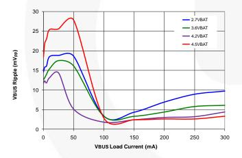
Figure 29. Output Ripple vs. V<sub>BAT</sub>
