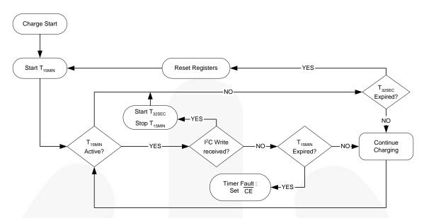
Figure 41. Timer Flow Chart for FAN5400, FAN5402, FAN5403, FAN5405
