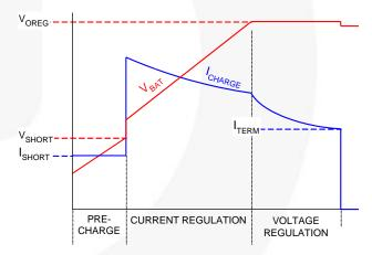
Figure 36. Charge Curve, I<sub>INLIM</sub> Limits I<sub>CHARGE</sub>
