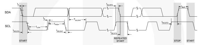
Figure 5. I<sup>2</sup>C Interface Timing for Fast and Slow Modes
