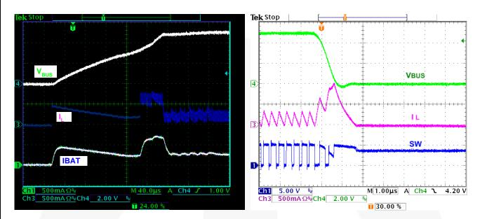
Figure 31. Startup, 3.6  $V_{BAT},$  44  $\Omega$  Load, Additional 10  $\mu F,$  X5R Across  $V_{BUS}$
