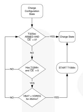
Figure 39. Charge Configuration
