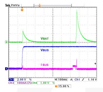
Figure 17. No Battery at V<sub>BUS</sub> Power-up; FAN5400, FAN5403
