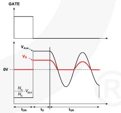
Figure 36. Waveforms for Line Voltage Detection
