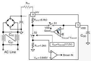
Figure 43. HV Startup Circuit
