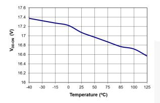
Figure 5. Turn-On Threshold Voltage (V<sub>DD-ON</sub>) vs. Temperature
