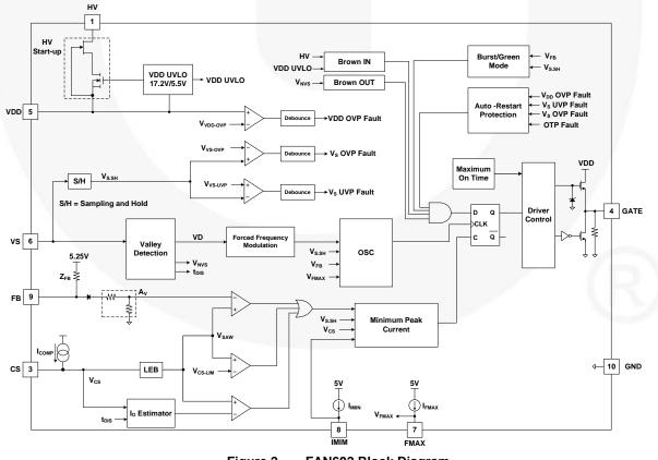
Figure 2. FAN602 Block Diagram
