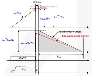
Figure 40. Effect of MOSFET Turn-off Delay
