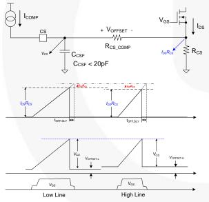
Figure 41. Line Voltage Compensation
