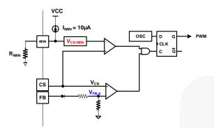
Figure 31. IMIN Function Circuit
