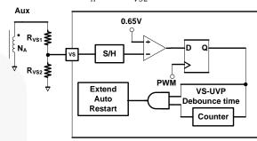
Figure 48. VS-UVP Protection Circuit
