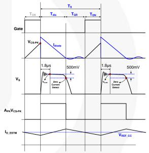
Figure 39. Waveforms for Estimate Output
