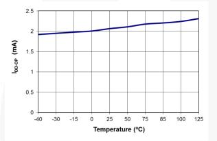
Figure 7. Operating Supply Current (I<sub>DD-OP</sub>) vs. Temperature
