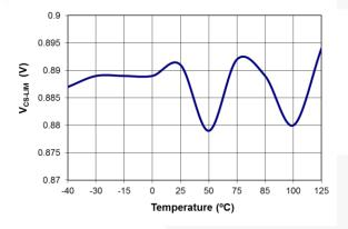
Figure 21. Current Limit Threshold Voltage (V<sub>CS-LIM</sub>) vs. Temperature
