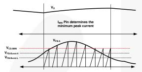
Figure 32. Burst-Mode Operation with IMIN
