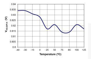
Figure 17. Output Under-Voltage Protection (V<sub>VS-UVP-H</sub>) vs. Temperature
