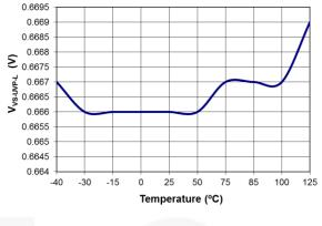
Figure 18. Output Under-Voltage Protection (V<sub>VS-UVP-L</sub>) vs. Temperature
