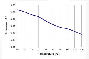
Figure 19. Maximum Current Sense Voltage (V<sub>CS-IMIN-MAX</sub>) vs. Temperature
