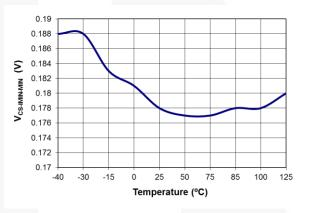
Figure 20. Minimum Current Sense Voltage (V<sub>CS-IMIN-MIN</sub>) vs. Temperature
