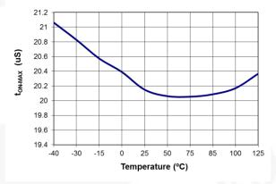
Figure 22. Maximum On Time (t<sub>ON-MAX</sub>) vs. Temperature
