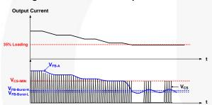
Figure 33. System enter Burst-mode Behavior
