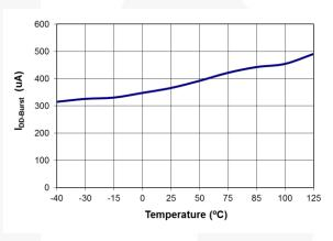
Figure 8. Burst-Mode Operating Supply Current (I<sub>DD-Burst</sub>) vs. Temperature
