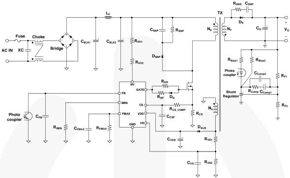
Figure 1. FAN602 Typical Application
