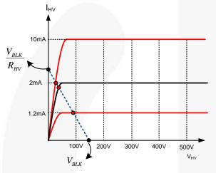
Figure 44. Characteristics of HV pin
