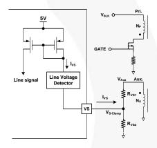
Figure 35. Line Voltage Detection Circuit
