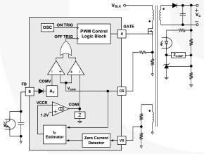
Figure 37. Simplified PWM Control Circuit
