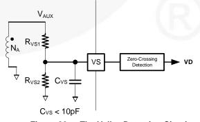
Figure 26. The Valley Detection Circuit
