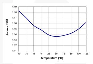
Figure 13. Frequency Fold-back Stopping (V<sub>FB-BNK-L</sub>) vs. Temperature
