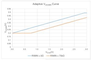
Figure 34.  $V_{\text{CS-IMIN}}$  as a Function of R<sub>IMIN</sub> with Variation of V<sub>S-SH</sub>
