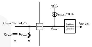
Figure 24. FMAX Function Circuit
