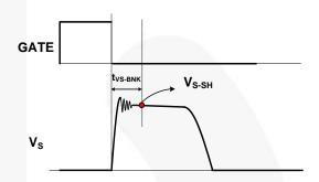
Figure 30. Output Voltage Detection
