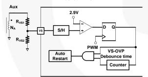
Figure 47. VS-OVP Protection Circuit
