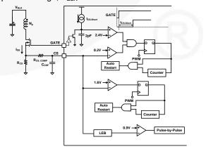
Figure 49. Current Sense Protection Circuit
