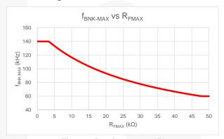
Figure 25. f<sub>BNK-MAX</sub> vs. R<sub>FMAX</sub>
