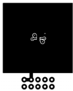
c. 69^\circ\text{C/W} when mounted on a 1 in 2 pad of 2 oz copper.
