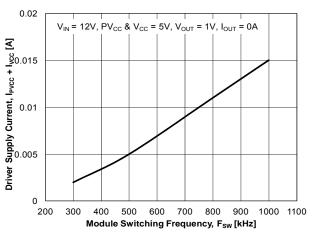
Figure 13. Driver Supply Current vs. Switching Frequency
