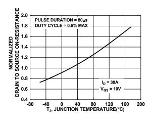
Figure 12. Normalized R<sub>DSON</sub> vs. Junction Temperature
