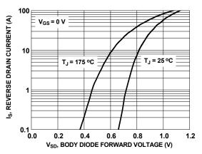
Figure 8. Forward Diode Characteristics
