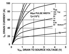
Figure 10. Saturation Characteristics
