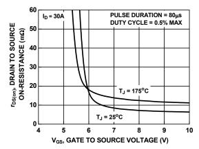
Figure 11. R<sub>DSON</sub> vs. Gate Voltage
