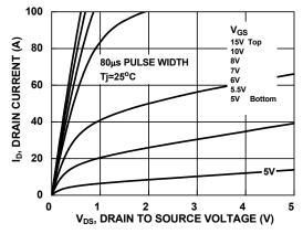
Figure 9. Saturation Characteristics
