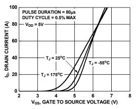
Figure 7. Transfer Characteristics
