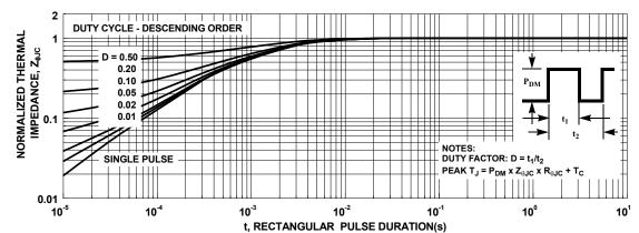
Figure 3. Normalized Maximum Transient Thermal Impedance
