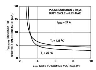
Figure 6. On-Resistance vs Gate to **Source Voltage**
