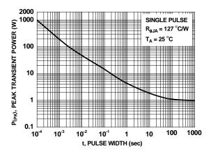
Figure 12. Single Pulse Maximum Power Dissipation
