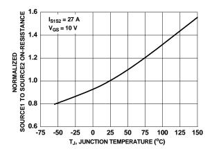
Figure 5. Normalized On-Resistance vs Junction Temperature
