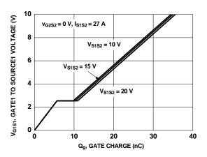
Figure 9. Gate Charge Characteristics
