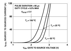
Figure 7. Transfer Characteristics
