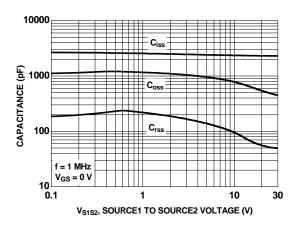
Figure 10. Capacitance vs Source1 to Source2 Voltage
