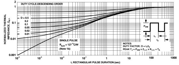
Figure 13. Junction-to-Ambient Transient Thermal Response Curve
