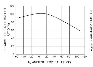
Figure 3. Relative Current Ratio vs. Ambient Temperature
