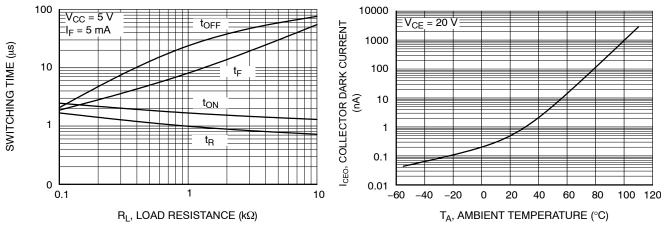
Figure 7. Switching Time vs. Load Resistance
