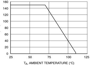
Figure 10. Max Allowable Power Dissipation (Detector) vs. Ambient Temperature
