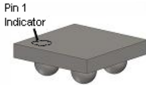
Figure 3. WLCSP Bumps Facing Down (Top View)
