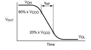
$$I_{OLD} \approx (C_L + C_{I/O}) \times \frac{\Delta V_{OUT}}{\Delta t} = (C_L + C_{I/O}) \times \frac{(80\% - 20\%) \bullet V_{CCO}}{t_{FALL}}$$
