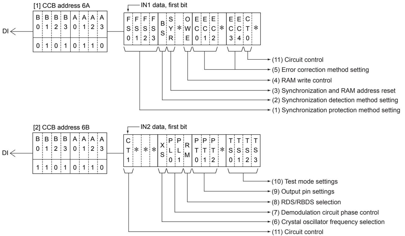
Caution : The bits labeled with an asterisk must be set to 0.
