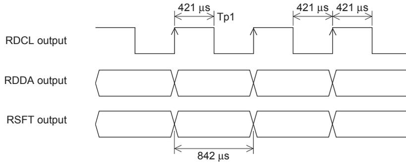
Note : When  $PT2 = 0$ , RDDA and RSFT must be acquired on the falling edge of RDCL.
