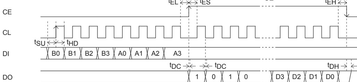
Cautions : 1. Since the DO pin is an n-channel open-drain output, the transition times ( $t_{DC}$ ,  $t_{DH}$ ) will differ with the value of the pull-up resistor used.
