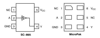
Figure 1. Pinout Diagrams (Top Views)
