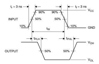
Figure 5. AC Waveforms
