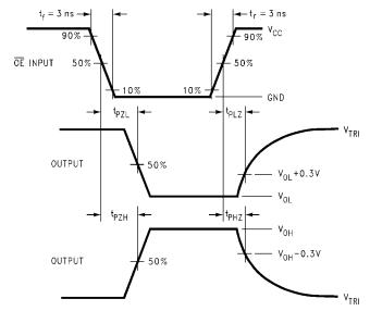
FIGURE 2. AC Waveforms
