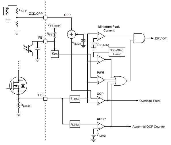
Figure 7. Current Sense Logic
