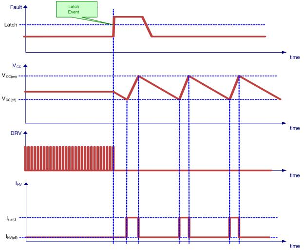
Figure 26. Latched Overload Operation
