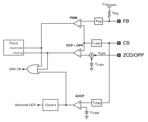
Figure 25. Overload Circuitry
