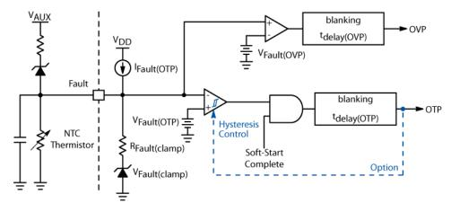
Figure 24. Fault Pin Internal Schematic
