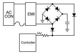
Figure 4. High–Voltage Input Connection
