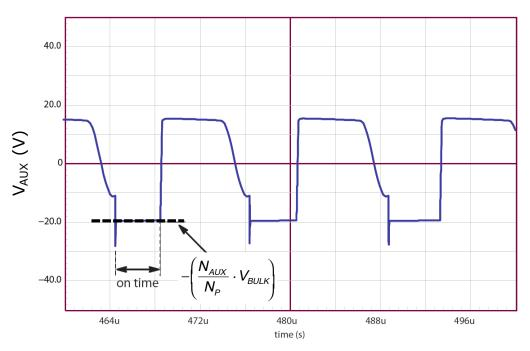
Figure 9. Auxiliary Winding Voltage
