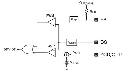
Figure 8. OPP Circuit Schematic
