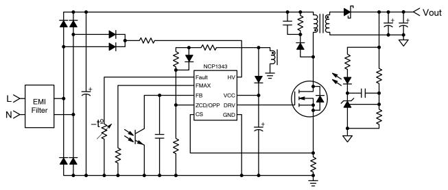
Figure 2. NCP1343 9–Pin Typical Application Circuit
