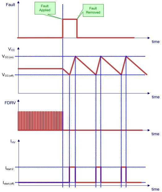
Figure 20. Operation During Latching Fault
