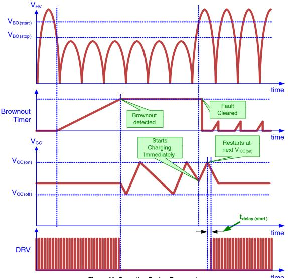
Figure 23. Operation During Brownout
