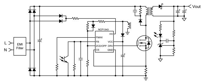
Figure 1. NCP1343 8–Pin Typical Application Circuit
