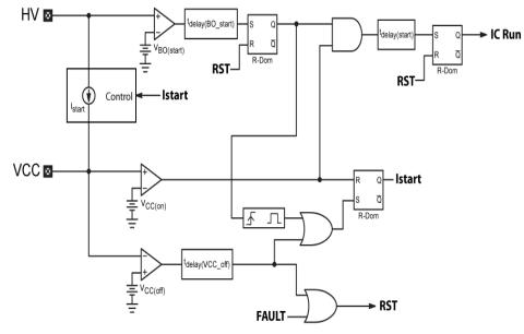
Figure 5. Start-up Circuitry Block Diagram
