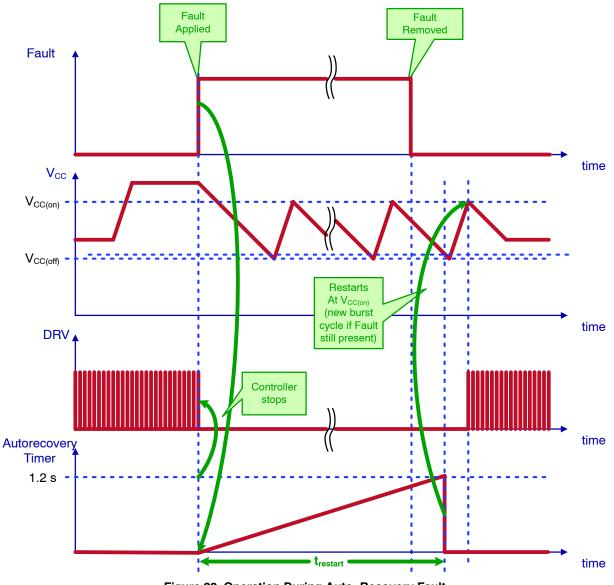
Figure 22. Operation During Auto-Recovery Fault
