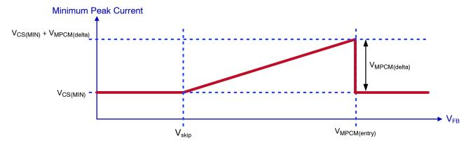
Figure 14. Minimum Peak Current Modulation
