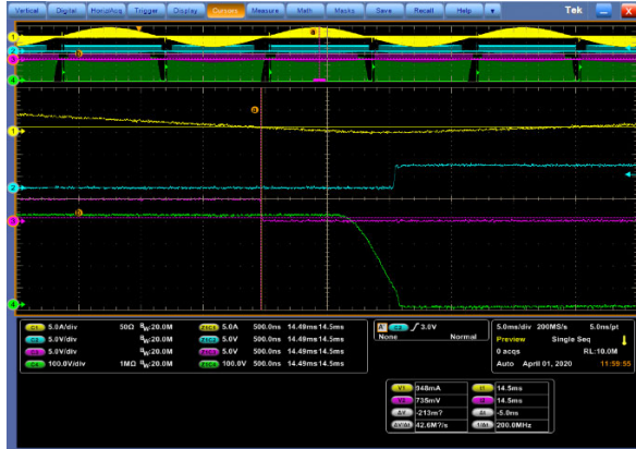
Figure 27. Valley Detection in CrM. Positive Half Line Cycle on Left, Negative on Right
