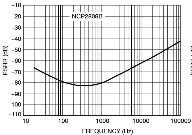
**Figure 34. PSRR – Input Grounded with  $10\ \Omega$**
