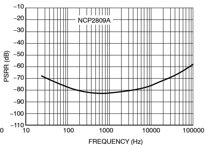
**Figure 29. PSRR – Input Grounded with  $10 \Omega$**
