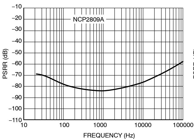
**Figure 30. PSRR – Input Grounded with  $10\ \Omega$**
