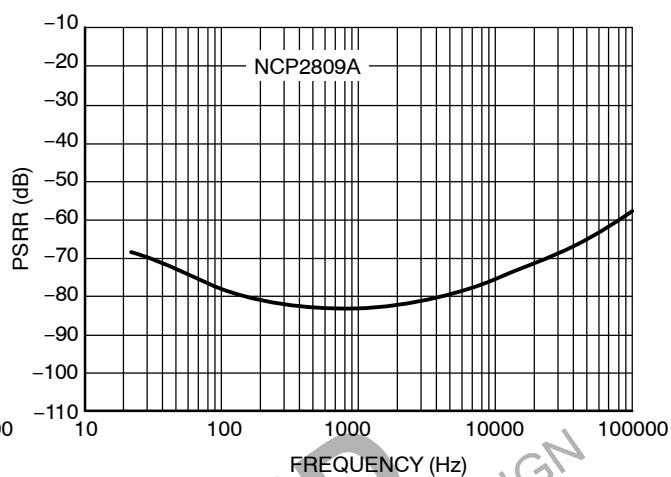
**Figure 31. PSRR – Input Grounded with  $10\ \Omega$**
