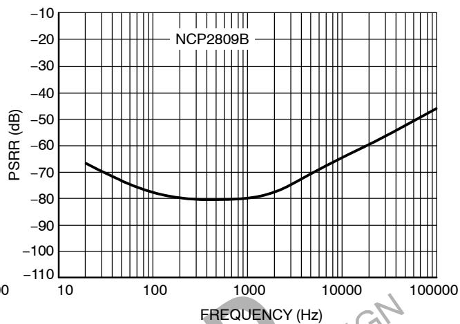
**Figure 35. PSRR – Input Grounded with  $10\ \Omega$**
