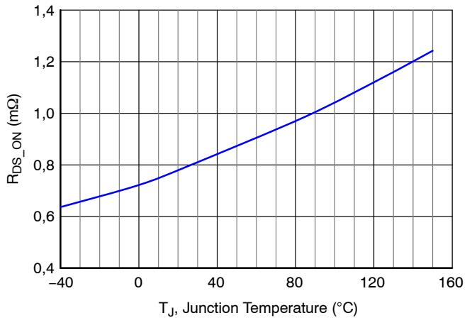
Figure 13. Low-Side R<sub>DS\_ON</sub> vs. Temperature, 5 V<sub>GS</sub>
