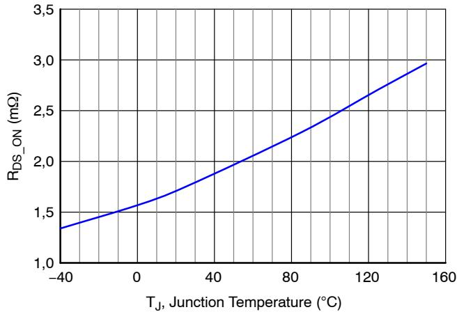
Figure 12. High-Side R<sub>DS\_ON</sub> vs. Temperature, 5 V<sub>GS</sub>
