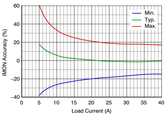
**Figure 25.** IMON Accuracy vs. Load
