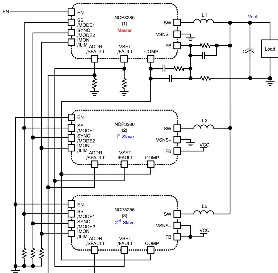
**Figure 4. Typical 120 A Application Circuit with 3 Parallel NCP3286**
