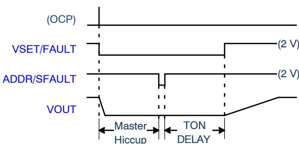
**Figure 36. Master/Slave Signals, Master OCP or UVP**
