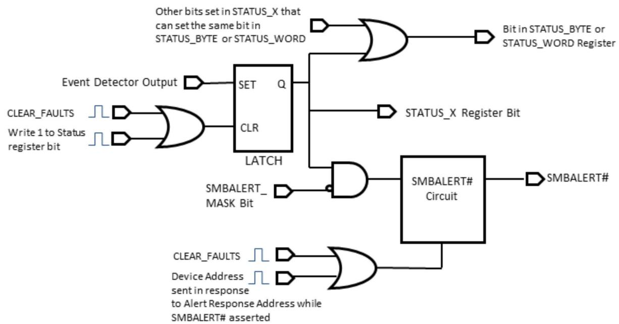
Figure 40. Status Bits and SMBALERT# Conceptual Schematic
