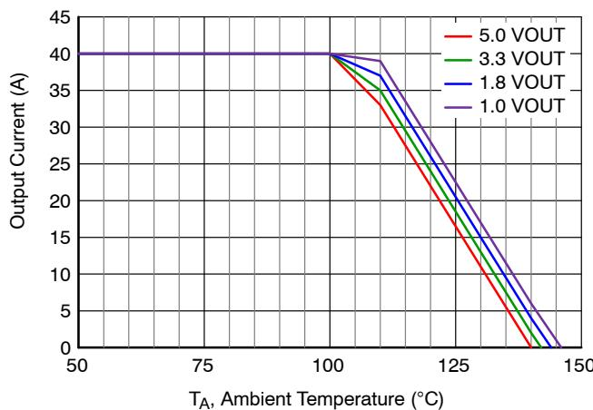
Figure 14. Thermal Safe Operating Area, No Airflow
