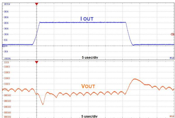
**Figure 20.** Load Transient Response, 1 – 21 A,
