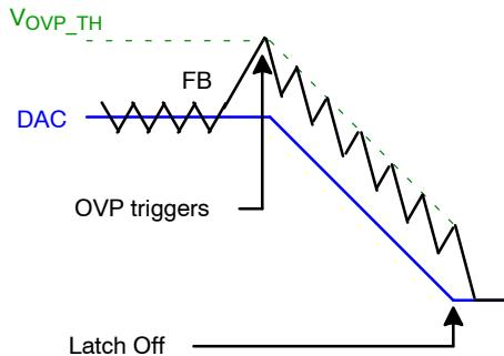
Figure 29. OVP Behavior during Normal Operation
