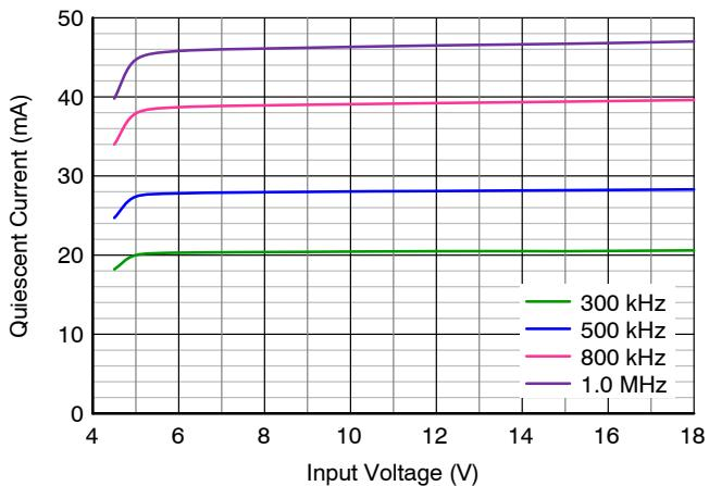
Figure 11. Device Quiescent Current vs. V<sub>IN</sub> and Frequency
