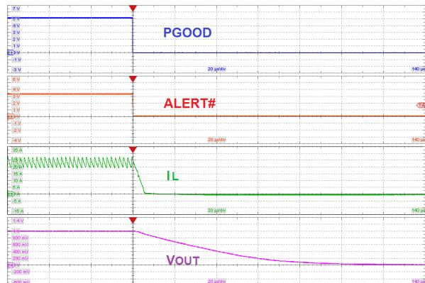
Figure 18. Over-Current Protection Response, Latch-Off,  $I_{LY} = 20$  A
