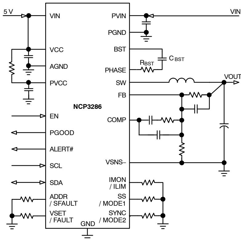
**Figure 2. Typical 12 V<sub>IN</sub>, 40 A Application Circuit with External 5 V VCC Supply (LDO Disabled)**
