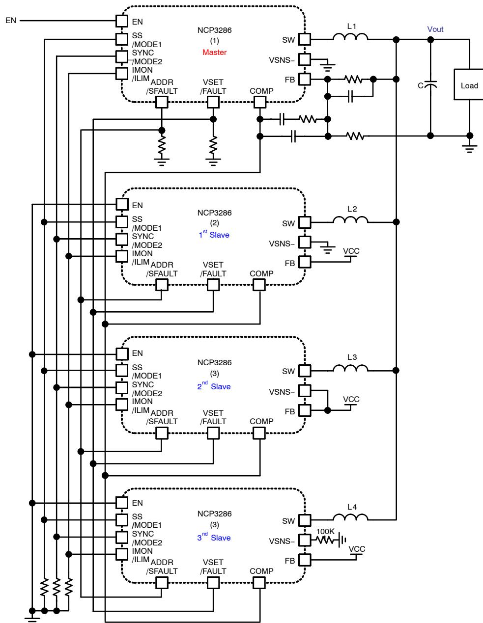
Figure 5. Typical 160 A Application Circuit with 4 Parallel NCP3286
