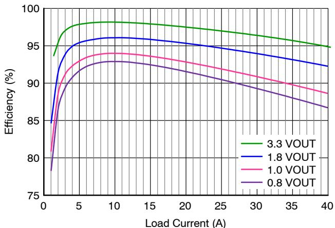
Figure 9. Efficiency vs. Load, 5 V<sub>IN</sub>, R<sub>BST</sub> = 0 Ω
