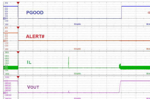
Figure 19. Over-Current Protection Response and Auto-Restart, Hiccup,  $I_{LY} = 20$  A
