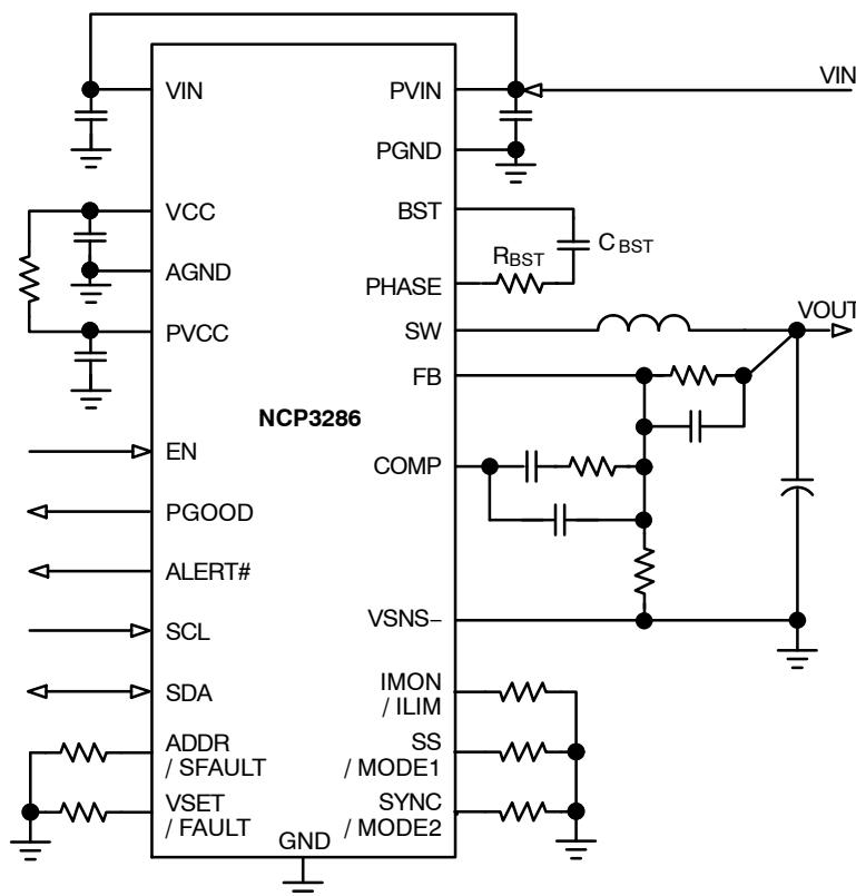
**Figure 1. Typical 12 V<sub>IN</sub>, 40 A Application Circuit for Single Input Supply (LDO Enabled)**
