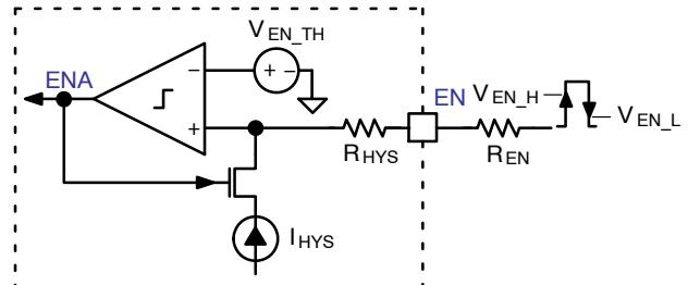
**Figure 26. Enable Thresholds and Hysteresis**
