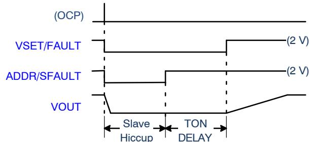
**Figure 37. Master/Slave Signals, Slave OCP or OT Fault**
