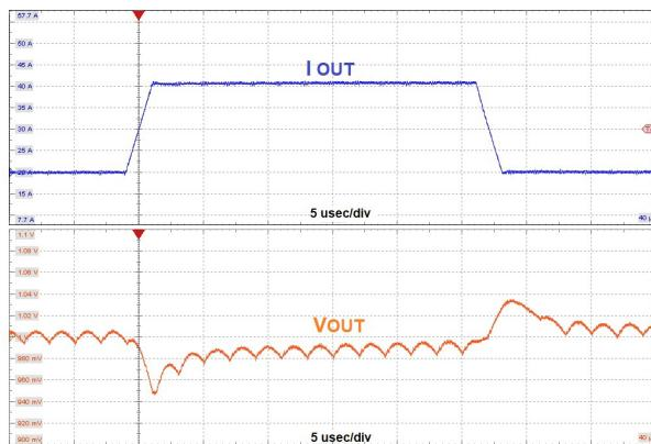
**Figure 21.** Load Transient Response, 20 – 40 A,
