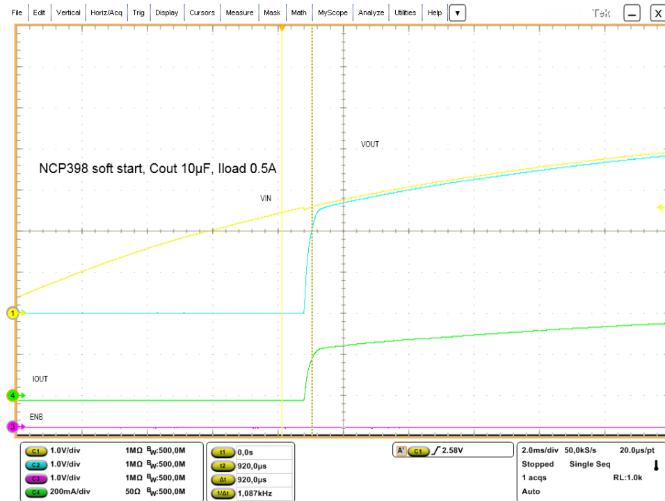
Figure 12. Soft Start On Cout 10 µF, 500 mA, Vin: yellow, Vout: blue, \overline{\text{EN}} : pink, IOUT: green
