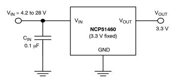
**Figure 1. Typical Application Schematics**
