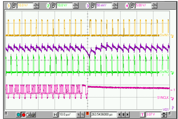
Top to Bottom: SWN_Slave, Vo_Slave, SWN_Master, Sync_clk Figure 13. From Sync to Unsync
