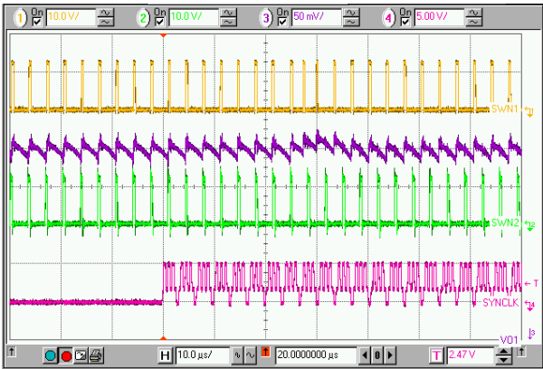
Top to Bottom: SWN_Slave, Vo_Slave, SWN_Master, Sync_clk Figure 12. From Unsync to Sync
