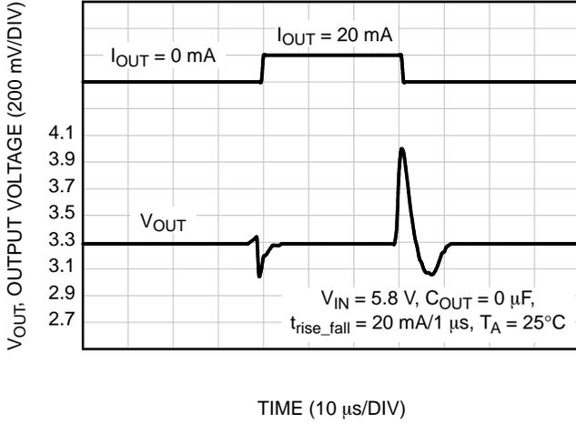
Figure 22. Load Transient Response 0 - 20 mA
