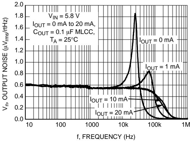
Figure 18. Output Voltage Noise 10 Hz - 1 MHz
