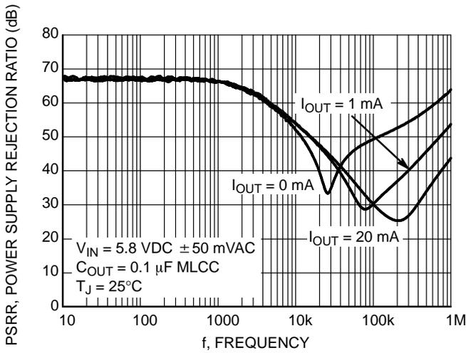
Figure 12. Power Supply Rejection Ratio
