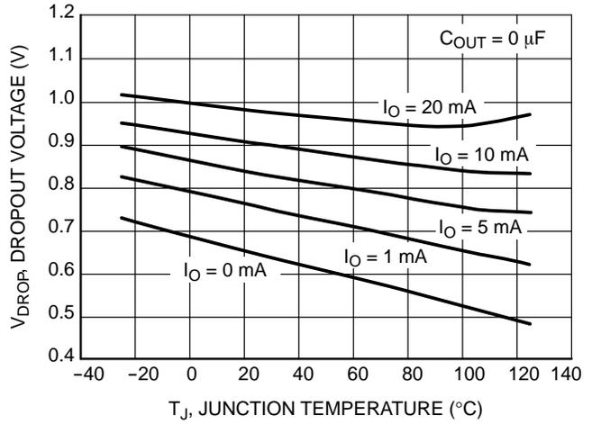
Figure 5. Dropout Voltage
