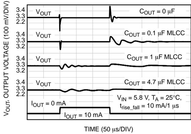
Figure 23. Load Transient Responses  $C_{OUT} = 0 - 4.7 \mu F$
