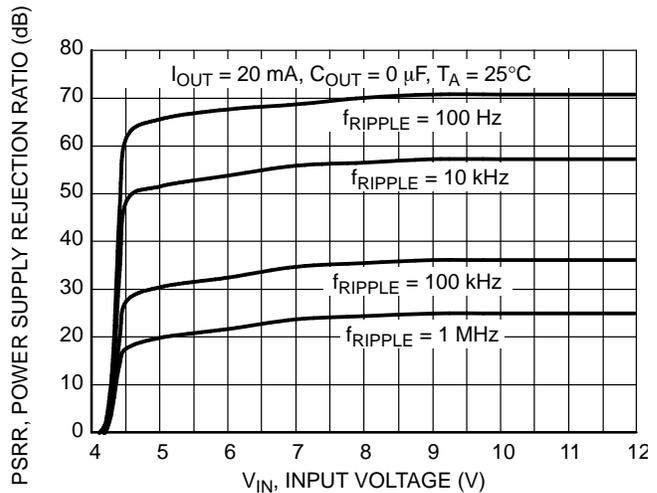
Figure 15. Power Supply Rejection Ratio vs. Input Voltage
