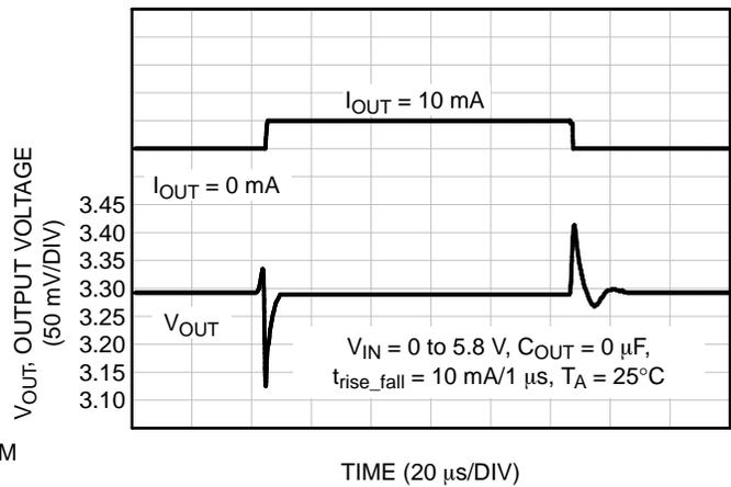
Figure 21. Load Transient Response 0 - 10 mA
