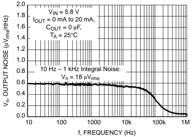
Figure 17. Output Voltage Noise 10 Hz - 1 MHz
