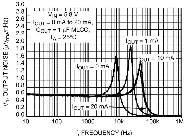
Figure 19. Output Voltage Noise 10 Hz - 1 MHz
