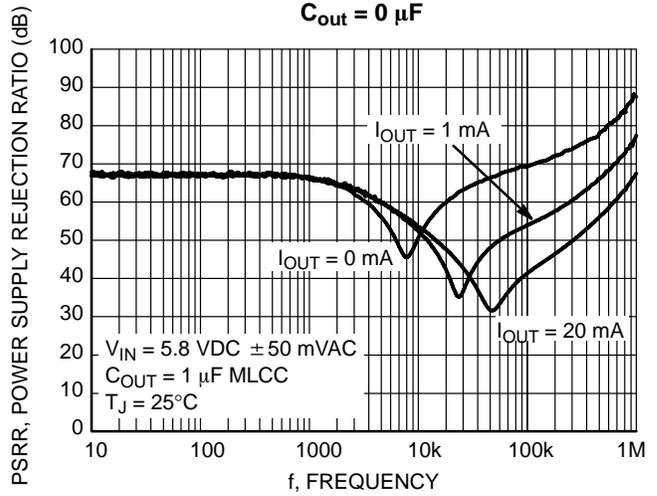
Figure 13. Power Supply Rejection Ratio
