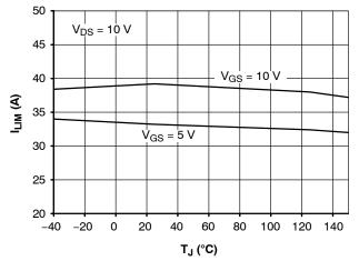
Figure 13. Current Limit vs. Junction Temperature
