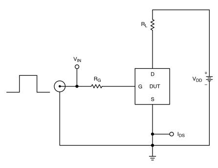
Figure 24. Resistive Load Switching Test Circuit
