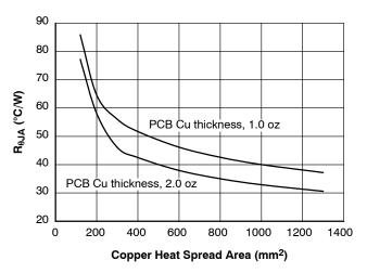
Figure 21.  $R_{\theta JA}$  vs. Copper Area
