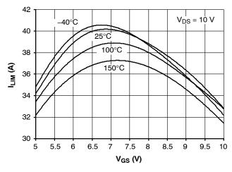
Figure 12. Current Limit vs. Gate-Source Voltage
