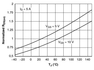
Figure 11. Normalized R<sub>DS(on)</sub> vs. Temperature
