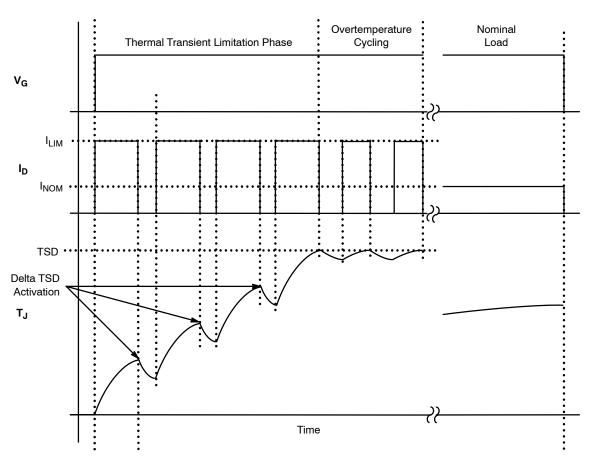
Figure 23. Overload Protection Behavior
