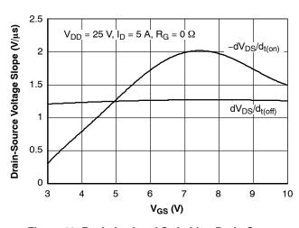
Figure 18. Resistive Load Switching Drain-Source Voltage Slope vs. Gate-Source Voltage
