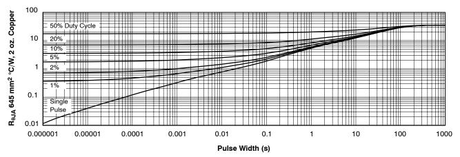
Figure 22. Transient Thermal Resistance
