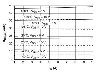
Figure 10. R<sub>DS(on)</sub> vs. Drain Current
