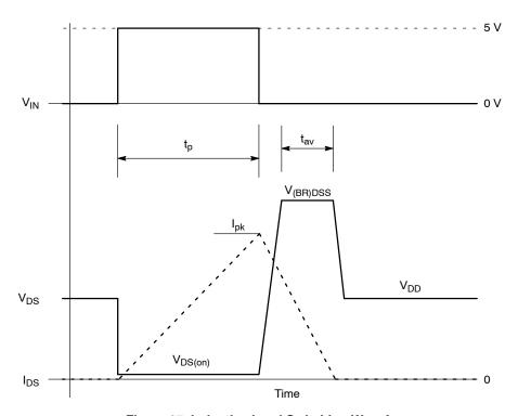
Figure 27. Inductive Load Switching Waveform
