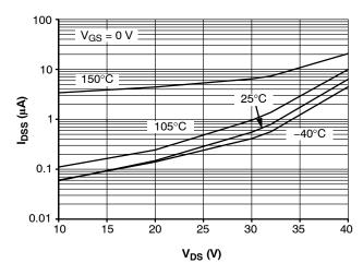
Figure 14. Drain-to-Source Leakage Current
