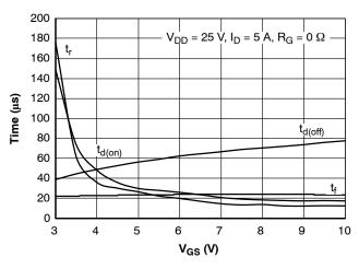
Figure 17. Resistive Load Switching Time vs.
