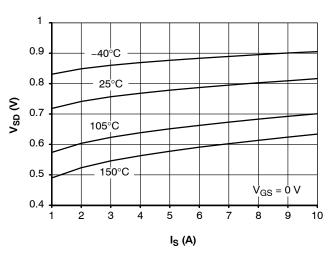
Figure 16. Source-Drain Diode Forward Characteristics
