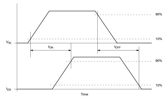
Figure 25. Resistive Load Switching Waveforms
