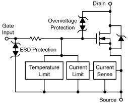
Figure 1. Block Diagram
