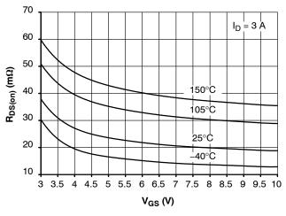
Figure 9. R<sub>DS(on)</sub> vs. Gate-Source Voltage
