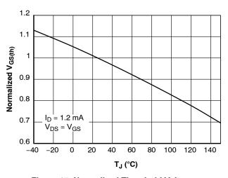
Figure 15. Normalized Threshold Voltage vs. Temperature
