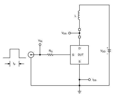
Figure 26. Inductive Load Switching Test Circuit
