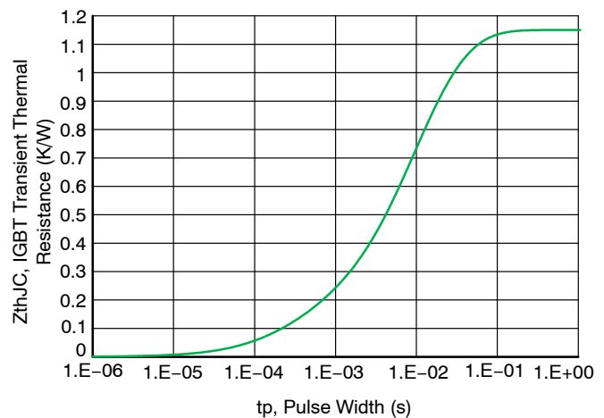
Figure 22. IGBT Transient Thermal Resistance
