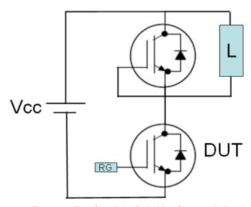
Figure 19. Test Circuit for Switching Characteristics
