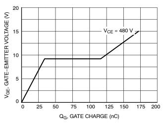
Figure 7. Typical Gate Charge
