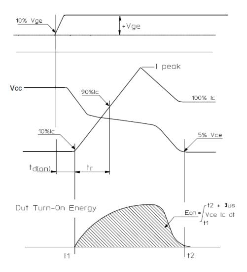
Figure 20. Definition of Turn On Waveform
