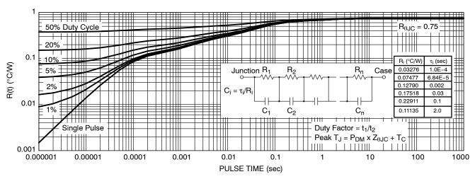
Figure 18. IGBT Transient Thermal Impedance
