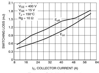
Figure 10. Switching Loss vs. I<sub>C</sub>
