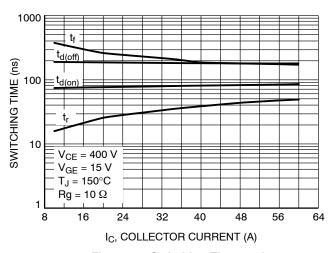
Figure 11. Switching Time vs. I<sub>C</sub>
