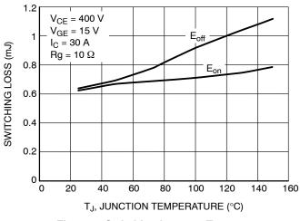
Figure 8. Switching Loss vs. Temperature
