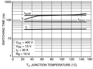
Figure 9. Switching Time vs. Temperature
