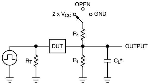
$C_L$  includes probe and jig capacitance
