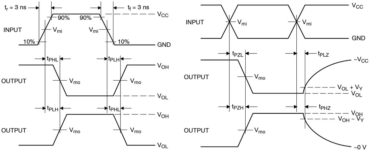
**Figure 4. Switching Waveforms**
