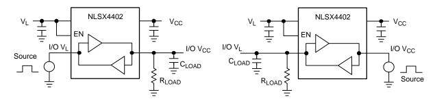
Figure 3. Rail–to–Rail Driving I/O  $V_L$ ,  $V_L$  to  $V_{CC}$
