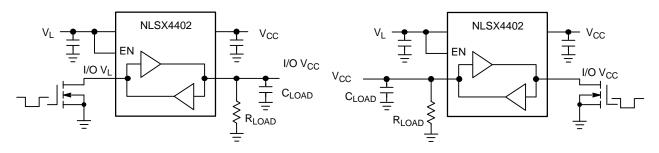
Figure 5. Open–Drain Driving I/O  $\rm V_L,$   $\rm V_L$  to  $\rm V_{CC}$
