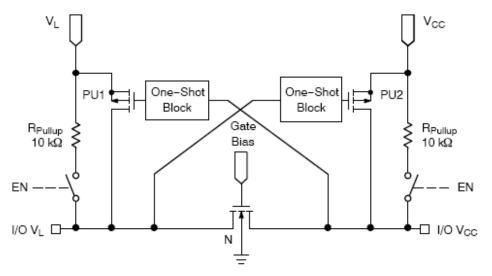
Figure 1. Block Diagram (1 I/O Line)
