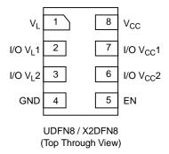
Figure 2. Pinout Diagram
