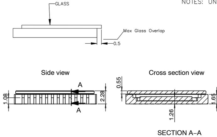
Figure 50. Package Drawing for the 48-pin LCC Package
