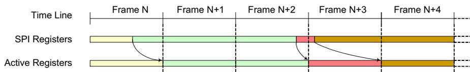
**Figure 20. Frame Synchronization of Configurations (no freezing)**
