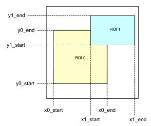
Figure 27. Overlapping Multiple Window Configuration
