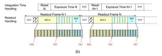
Figure 31. P1-SN/SE/FN, P3-SN/SE/FN: Frame Sync Codes
