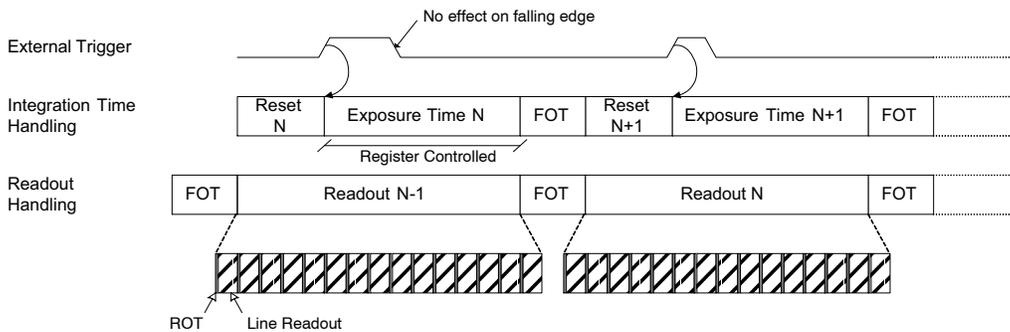
**Figure 14. Triggered Shutter Operated in Master Mode**
