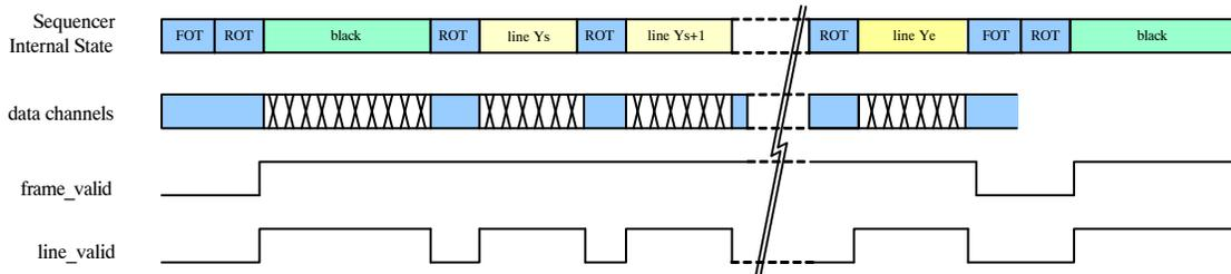
Figure 45. P2-SN/SE/FN: Frame Timing Indication
