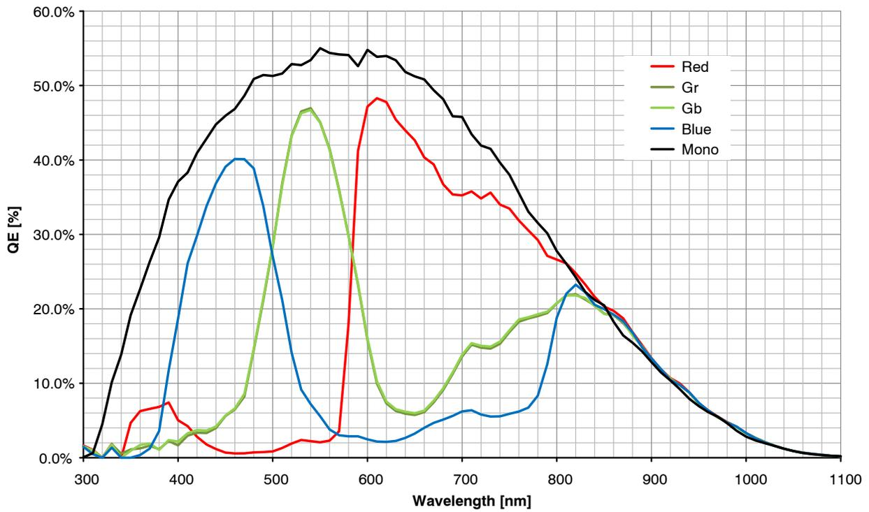
Figure 3. Quantum Efficiency Curve for Mono and Color
