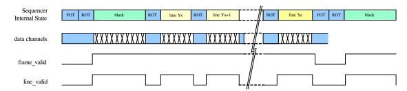
Figure 45. P2-SN/SE/FN: Frame Timing Indication
