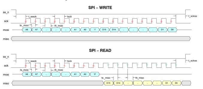
Figure 22. SPI Read and Write Timing Diagram
