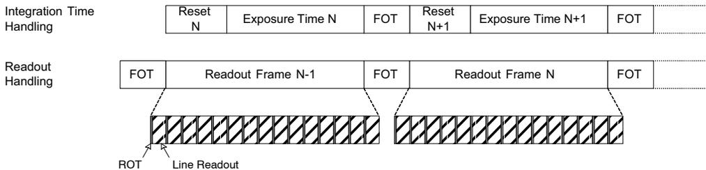
Figure 12. Integration and Readout for Pipelined Shutter
