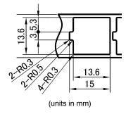
Figure 56. Dimensions of the Protective Foil
