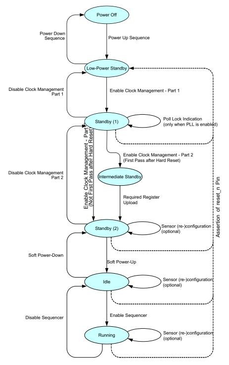
Figure 17. Sensor Operation Flowchart
