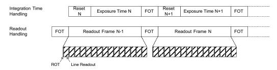
Figure 12. Integration and Readout for Pipelined Shutter
