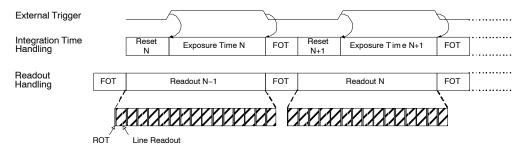
Figure 13. Pipelined Shutter Operated in Slave Mode
