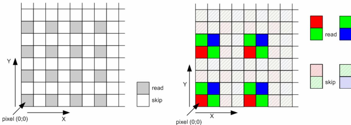
Figure 29. Subsampling Scheme for Monochrome and Color Sensors
