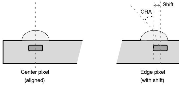
The center axes of the microlens and the photodiode coincide for the center pixels. For the edge pixels, there is a shift between the axes of the microlens and the photodiode causing a Peak Response Incidence Angle (CRA) that deviates from the normal of the pixel array.
