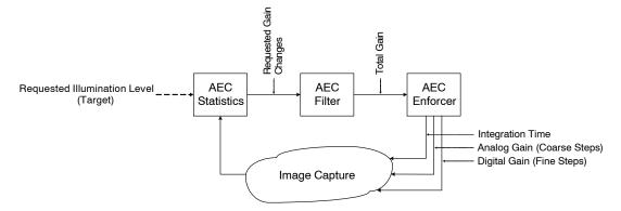
Figure 30. Automatic Exposure Control Loop
