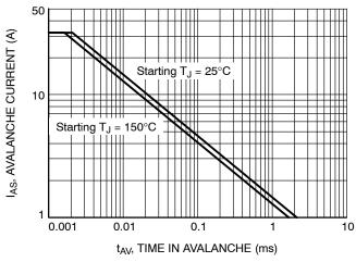
Figure 10. Unclamped Inductive Switching Capability
