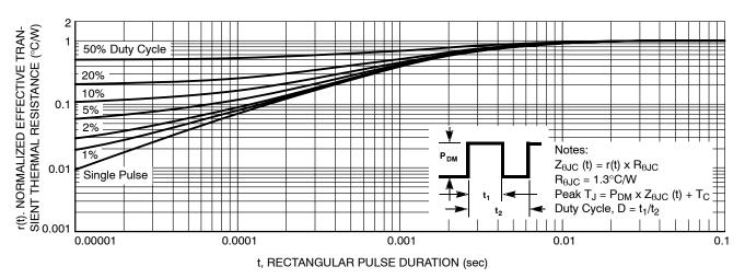
Figure 14. Junction-to-Ambient Thermal Response
