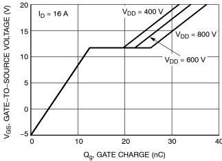
Figure 8. Gate-to-Source Voltage vs. Total Charge
