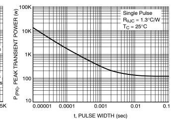
Figure 13. Single Pulse Maximum Power Dissipation
