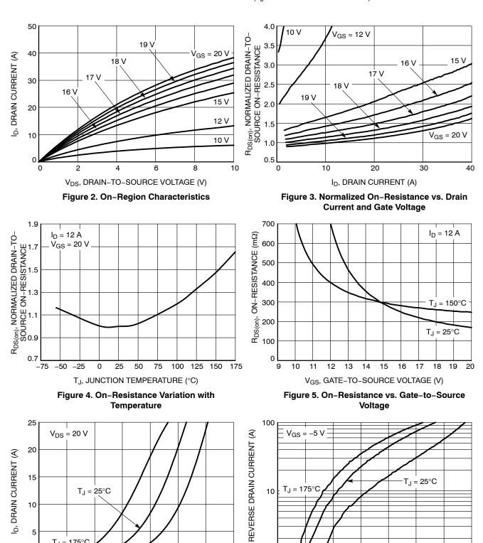
V<sub>GS</sub>, GATE-TO-SOURCE VOLTAGE (V) Figure 6. Transfer Characteristics
