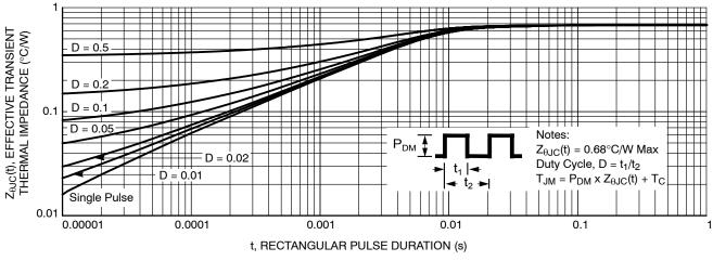
Figure 12. Transient Thermal Impedance
