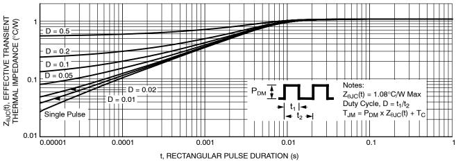
Figure 12. Transient Thermal Impedance
