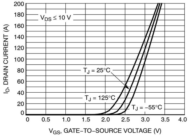
Figure 2. Transfer Characteristics
