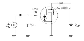
Fig.2 Switching Time Test Circuit
