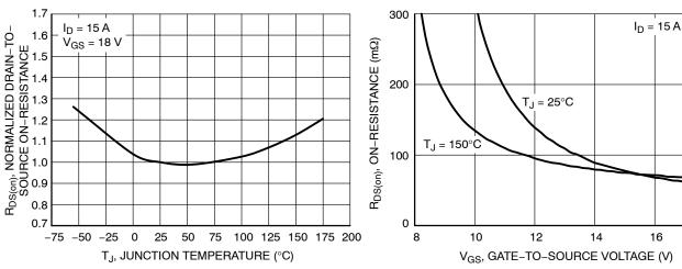
Figure 3. On-Resistance Variation with **Temperature**
