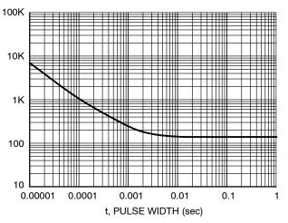
Figure 12. Single Pulse Maximum Power Dissipation
