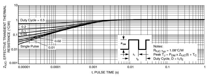
Figure 13. Junction-to-Case Transient Thermal Response
