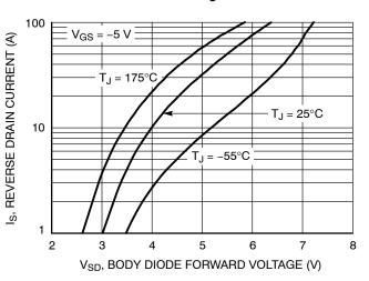
Figure 6. Diode Forward Voltage vs. Current
