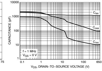
Figure 8. Capacitance vs. Drain-to-Source Voltage
