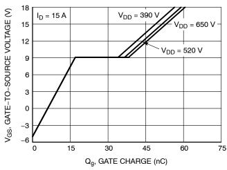
Figure 7. Gate-to-Source Voltage vs. Total Charge
