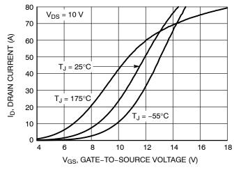
Figure 5. Transfer Characteristics
