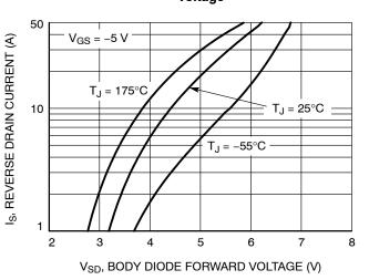
Figure 6. Diode Forward Voltage vs. Current
