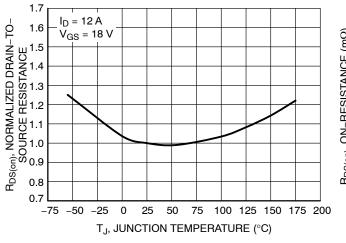
Figure 3. On–Resistance Variation with Temperature
