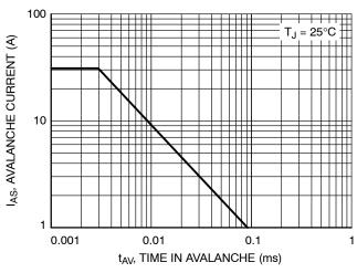
Figure 9. Unclamped Inductive Switching Capability
