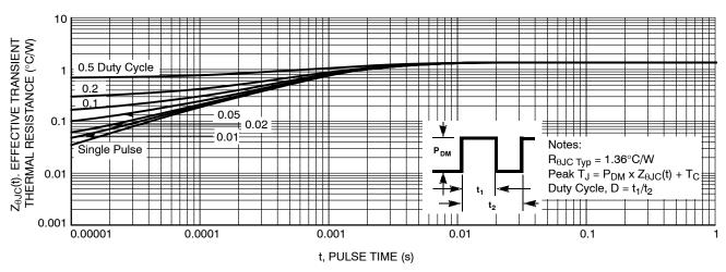
Figure 13. Junction-to-Case Thermal Response
