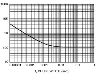
Figure 12. Single Pulse Maximum Power Dissipation
