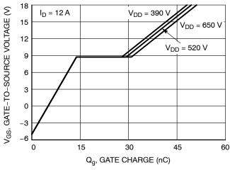
Figure 7. Gate-to-Source Voltage vs. Total Charge
