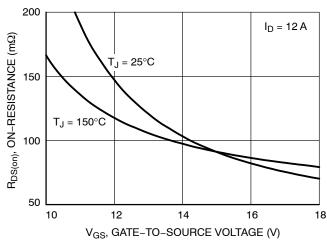
Figure 4. On-Resistance vs. Gate-to-Source Voltage
