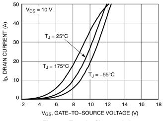
Figure 5. Transfer Characteristics
