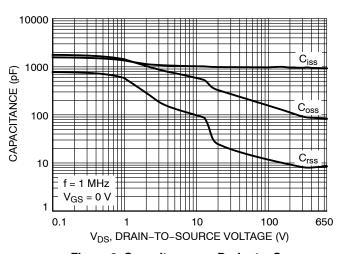
Figure 8. Capacitance vs. Drain-to-Source Voltage
