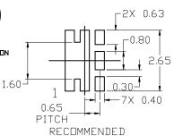
MOUNTING FOOTPRINT For additional information on our Pb-Free strategy and soldering details, please download the DN Seniconductor Soldering and Mounting Techniques Reference Manual, SDLDERRM/D.
