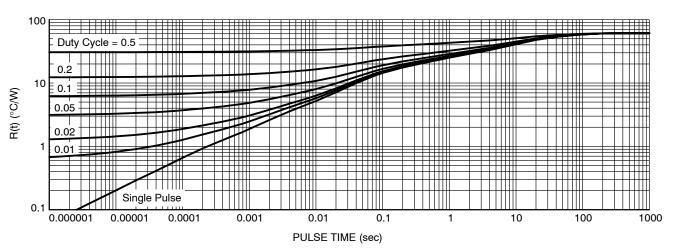
Figure 13. Transient Thermal Impedance
