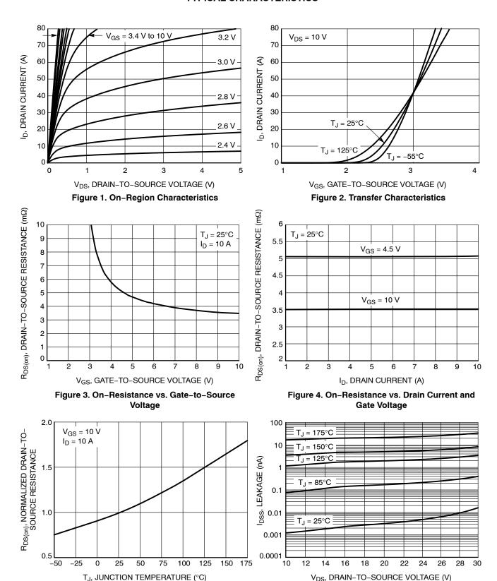
Figure 5. On–Resistance Variation with Temperature
