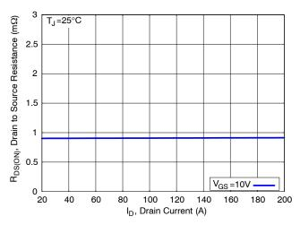
Figure 4. On-Resistance vs. Drain Current
