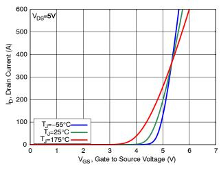
Figure 2. Transfer Characteristics
