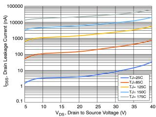
Figure 6. Drain Leakage Current vs. Drain Voltage
