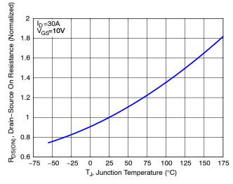
Figure 5. Normalized ON Resistance vs. Junction Temperature
