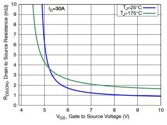
Figure 3. On-Resistance vs. Gate Voltage
