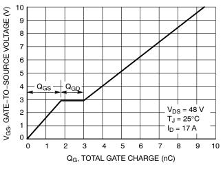
Figure 8. Gate-to-Source vs. Total Charge
