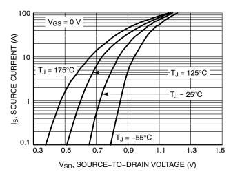
Figure 10. Diode Forward Voltage vs. Current
