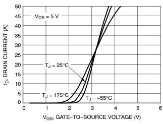
Figure 2. Transfer Characteristics
