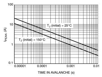
Figure 12. I<sub>PEAK</sub> vs. Time in Avalanche
