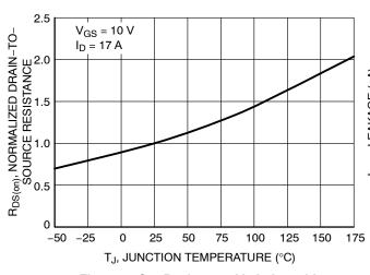
Figure 5. On–Resistance Variation with Temperature
