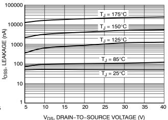
Figure 6. Drain-to-Source Leakage Current vs. Voltage
