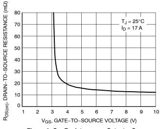
Figure 3. On-Resistance vs. Gate-to-Source Voltage
