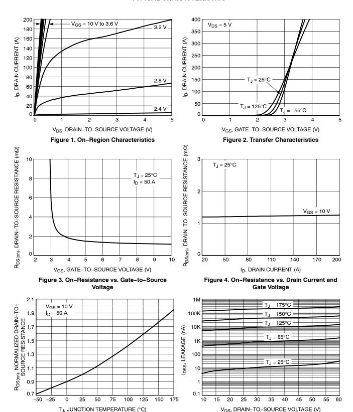
Figure 6. Drain-to-Source Leakage Current
