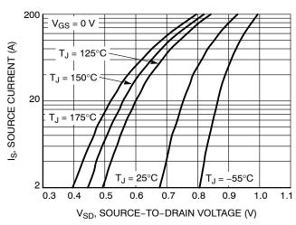
Figure 10. Diode Forward Voltage vs. Current
