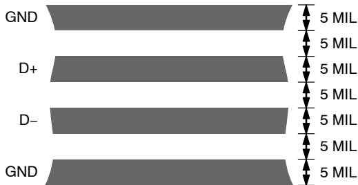
Figure 22. Typical Arrangement of Signal Tracks
