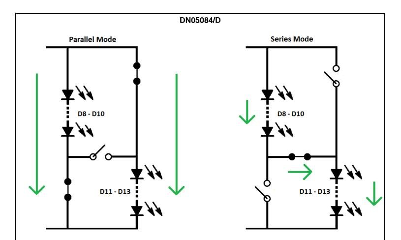
Figure 3 – The LED configuration is dynamically adjusted by the control circuitry depending on the instantaneous AC input voltage.
