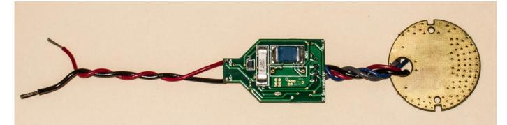
Figure 1 – Two-Stage Parallel-to-Series LED Lighting Circuit, with Switch-In CCR, available as evaluation board 40WBULBGEVB
