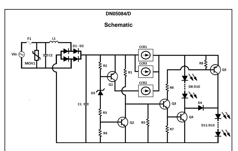
Figure 2 – Two-Stage Parallel-to-Series LED Lighting Circuit, with Switch-In CCR. It is possible to mount an inductor (L1) and a capacitor on the board for additional EMI filtering, but generally these are not needed. Inductor L1 has a 0 ohm resistor in its place on the evaluation board.
