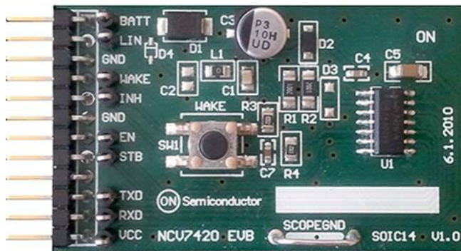
Figure 12. NCV7420EVB PCB Top Side View
