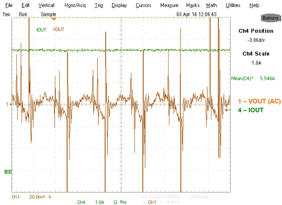
Figure 12. V_{IN} = 230 V_{AC} , I_{OUT} = 5.5 A , \Delta V_{OUTPK-PK} = 30 mV
