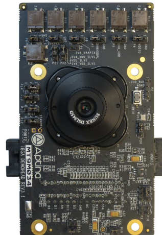
Figure 1. MT9M034 Evaluation Board
