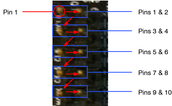
Figure 6. Pin Locations and Assignments of Grouped Jumpers. Pin 1 is Located at the Top-Left Corner and Increases in a Zigzag Fashion Shown in the Picture (P11 and P15 has different orientation)
